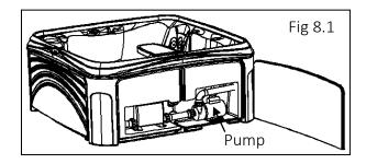
The pipes entering and leaving the pump are connected with large plastic unions. To purge the air from the pump, one of these unions will be slightly loosened.
