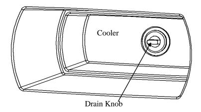
To drain the melt water from your cooler, turn the drain knob a couple of turns counterclockwise. Melt water will exit through the small hose located on the umbrella side, low by the lifter. This hose can be gently pulled out to help pour into a container. When done simply push the hose back into the cabinet until it hits the hose stop.
