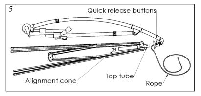
Ensuring the canopy's top side is out, fit the center hole of the canopy over the top tube of the cage assembly.
